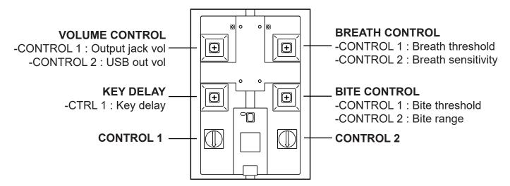
**Breath threshold**: While holding [PATCH SELECT] press the [OCTAVE UP] key. Turn [CONTROL KNOB 1] fully counter-clockwise. The [INDICATOR] LED will turn ON if the breath sensor is not being engaged, and OFF if it is. Increase the threshold until the [INDICATOR] LED on the back of the ZWI turns ON, and no sound is being produced.
